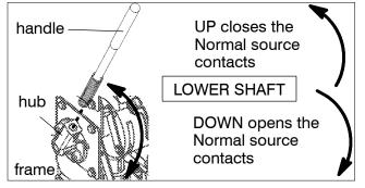
Figure 1-11. Normal (lower shaft) operation on 800–1200 amp. H–design transfer switches..
